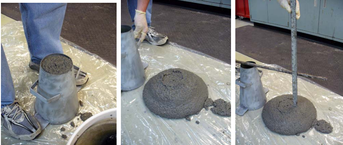
Figures 6-8: Filling the slump cone, cone removal, measurement of polymer concrete slump.
