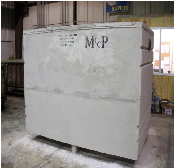
Precast vault before exterior coating
