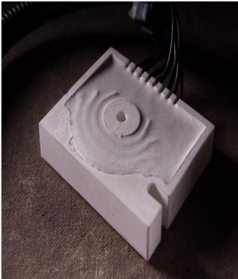
Potting wires in heating element ceramic base
